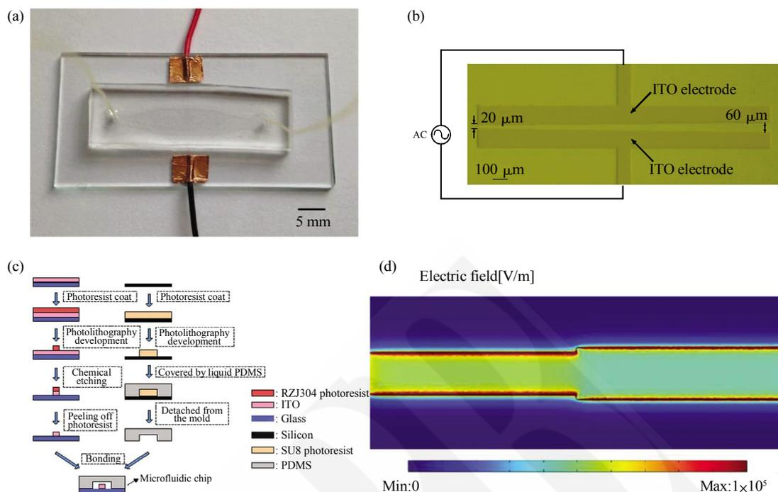
**Fig. 2 A microfluidic chip for cell electro-stretching**
