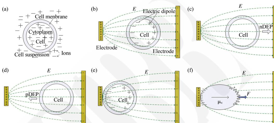
**Fig. 1 Model and DEP effect of a cell in suspension**
