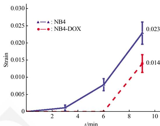
**Fig. 7 Strain versus time,  $t$  ( $0 < t < 3$  min:  $U = 2V_{pp}$ ;  $3 \text{ min} < t < 6$  min:  $U = 3V_{pp}$ ;  $6 \text{ min} < t < 9$  min:  $U = 4V_{pp}$ ), for NB4 and NB4-DOX cells, respectively**
