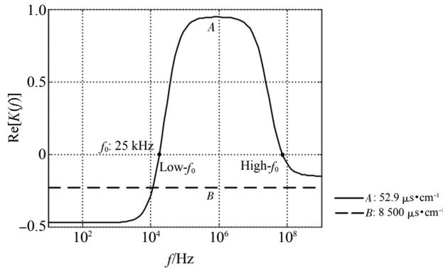
**Fig. 4 Real part of the polarization factor, Re[K(f)], versus frequency, f, at different conductivity of cell suspension  $\sigma_e$**
