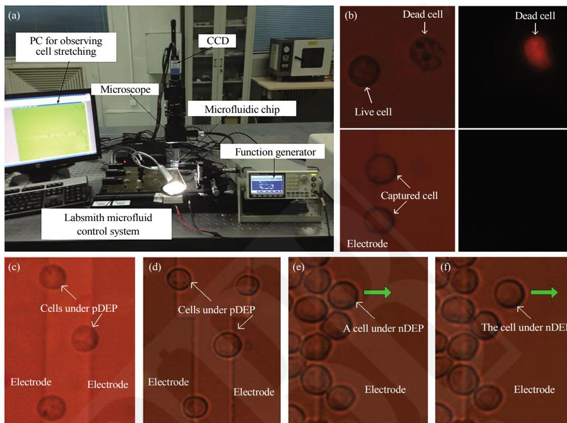
**Fig. 3 Cell DEP experiments and the viability testing of NB4 cells**
