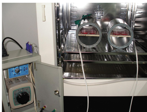
Fig. 1 The apparatus designed for treatment of cells by sinusoidal electromagnetic fields
