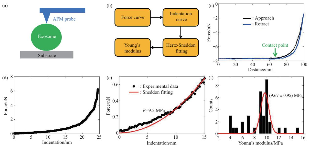
**Fig. 4** Measuring the Young's modulus of single living exosomes by AFM indentation assays
