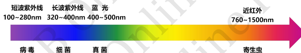
Fig. 2 Different wavelengths for inactivating various microorganisms
