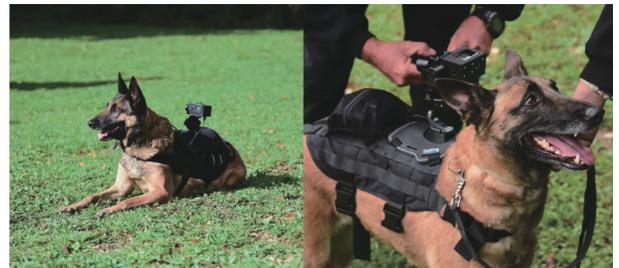
Fig. 5 K9 vest with RGB and thermal imaging camera<sup>[65]</sup>
