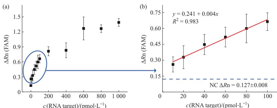
**Fig. 5 The sensitivity of DCPLP-RCA**
